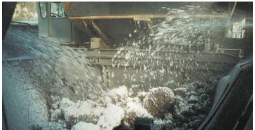
The foam suppression system at work in a mobile crusher.
