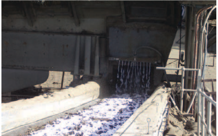
Polo BDS employs foam micro-bubbles at the application point and downstream.
